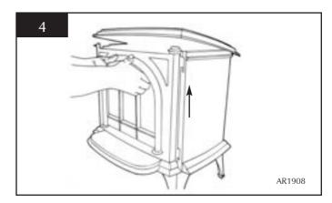
• Remove the glass frame by undoing the frame fixing screws and lifting clear, Diagram 5
